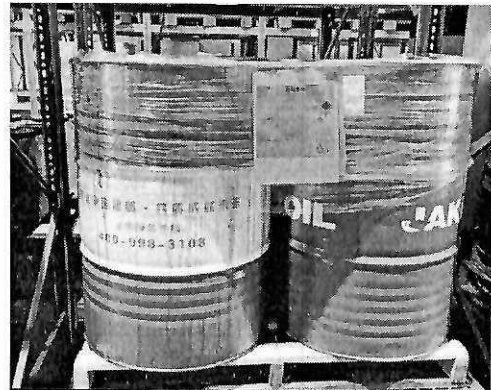
大金属桶类：标签彩打或橙色纸打印，托盘+缠绕膜打包，一托盘≤4桶
